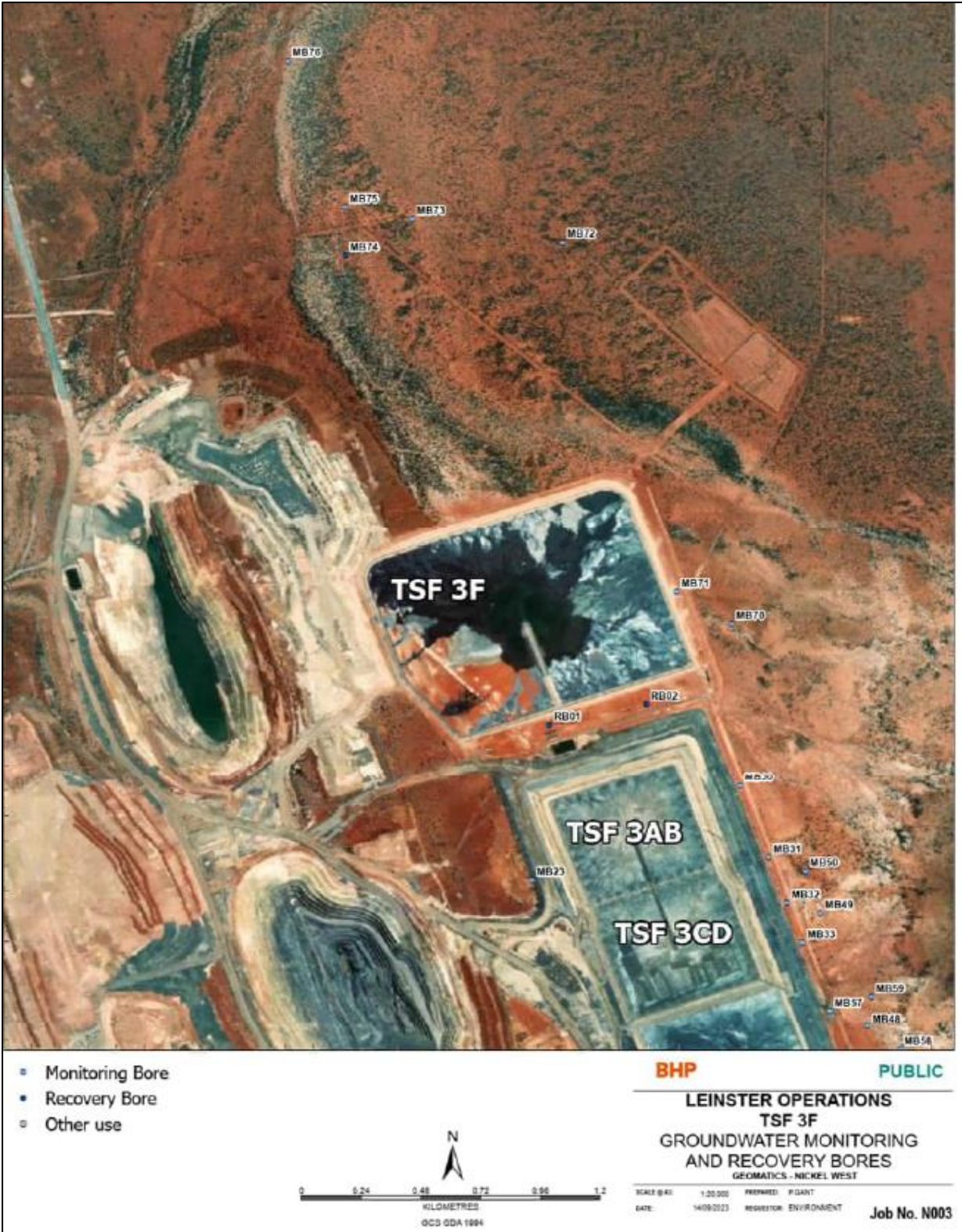
Figure 2: Groundwater monitoring bores around TSF3 Cell F and north of the proposed area for TSF3 Cell G.
