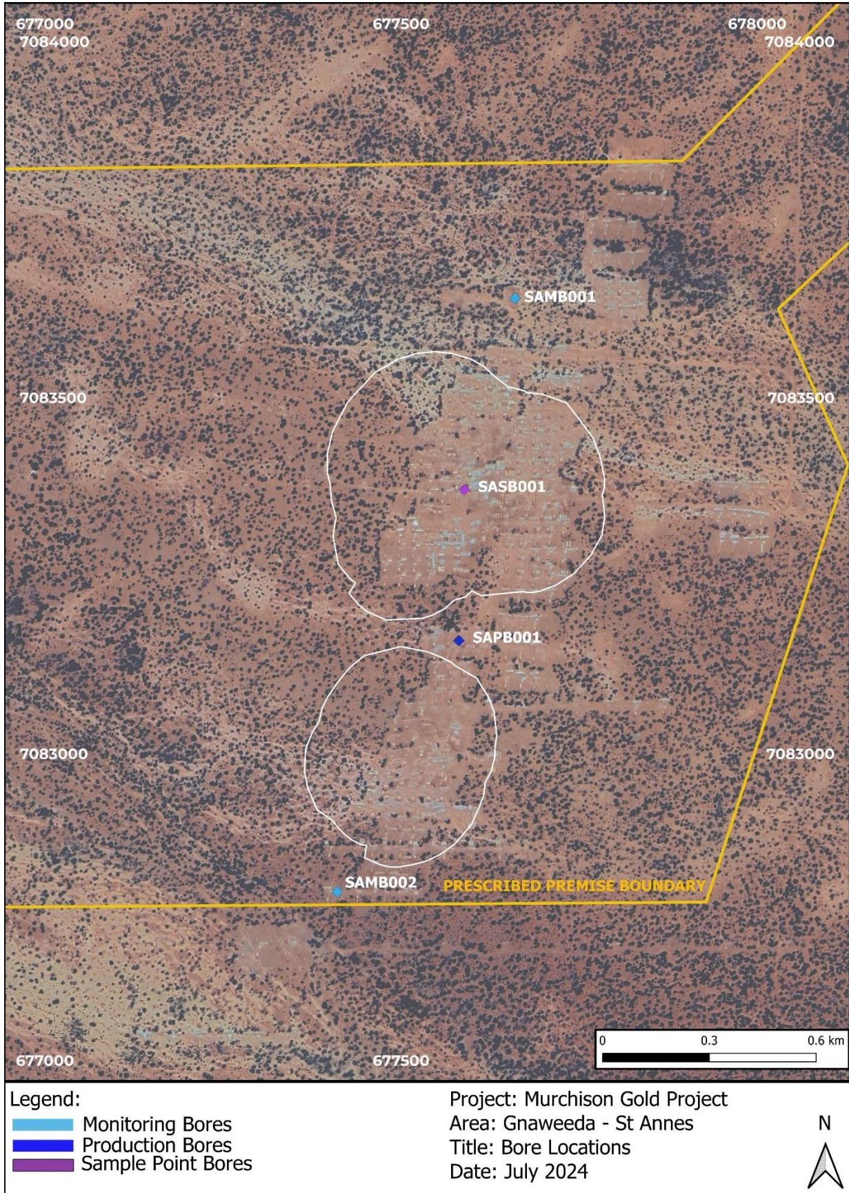
Figure 8: Bore locations in the St Annes Pit (SAMB001, SAMB002, and SAPB001 not constructed yet)
