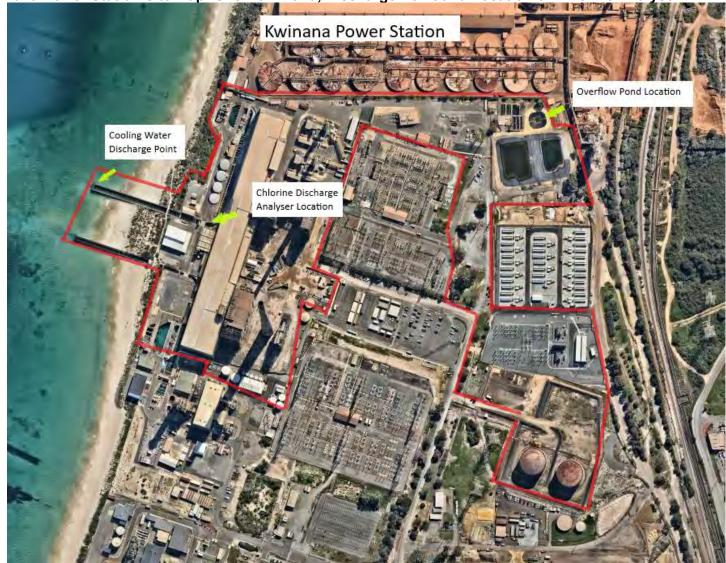
Attachment A. Kwinana Power Station Site Map: Overflow Pond, Discharge Point and Location of Chlorine Analyser
