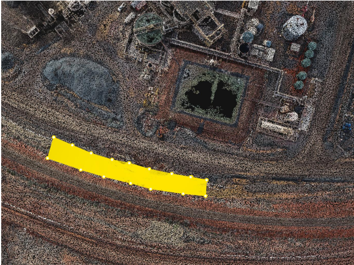
Figure 10: Map showing the 1000 m 2 extent of the tailings line 2 slurry discharge on M 37/25.
