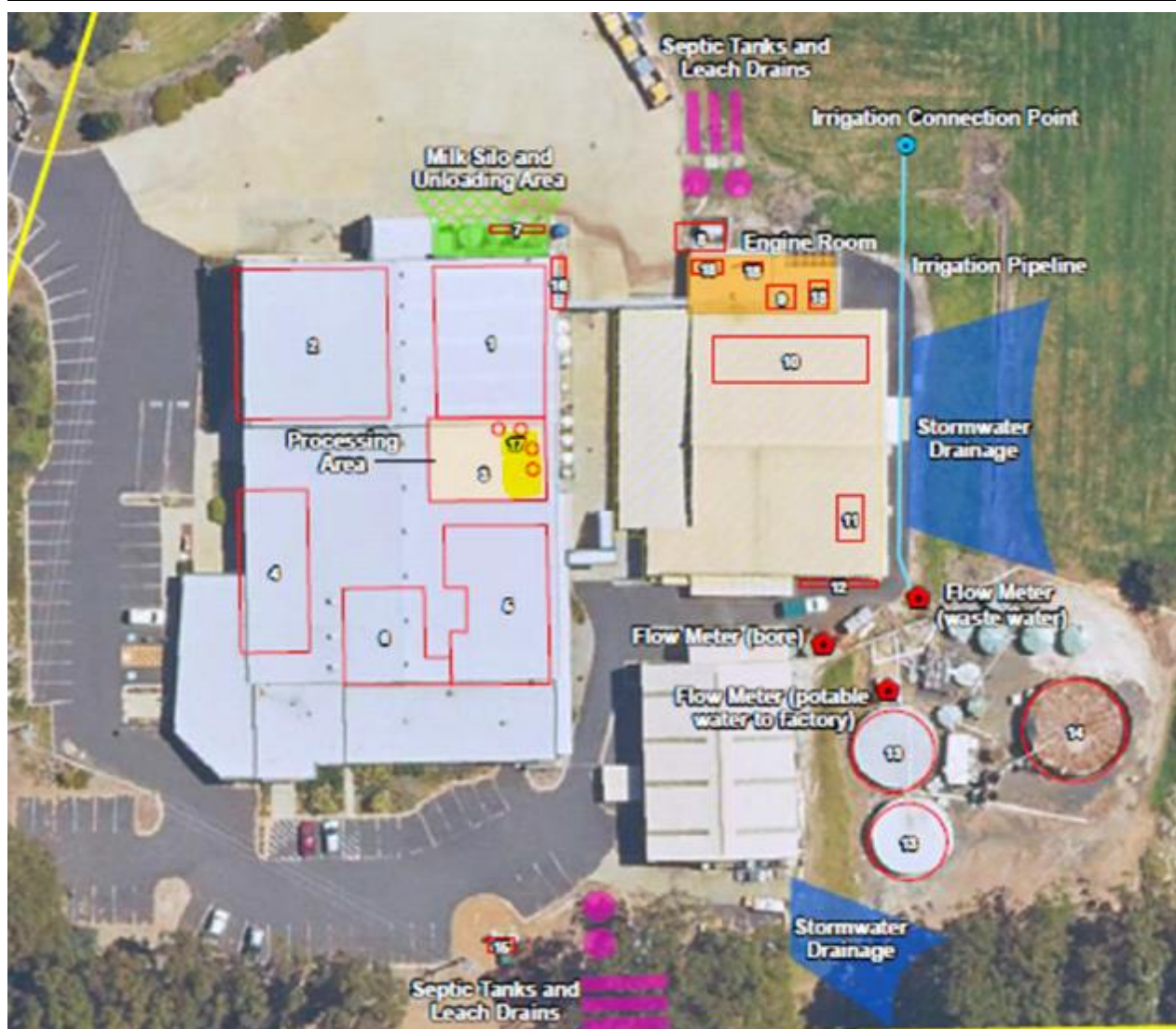
Figure 1. Highlighted in yellow (Yoghurt Holding Tank) – non-conforming yoghurt waste disposed into WWTP on 15/12/2021 causing the WWTS to overload resulting in slightly higher BOD level at 57 mg/L.
