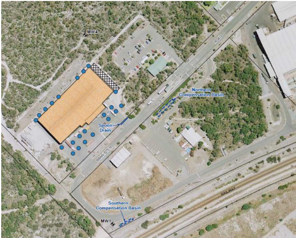
Figure 3: Premises stormwater drains and associated compensations basins.
