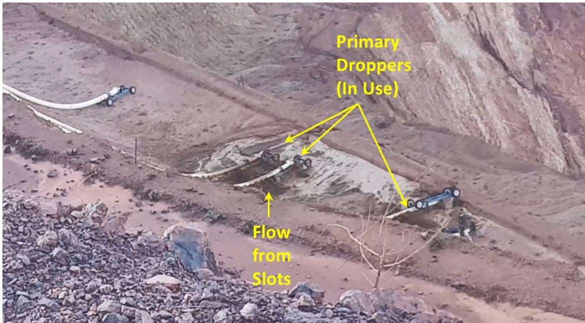
Figure I-4 View of Droppers from Near Manifold (3No. Primary Droppers Operating)
