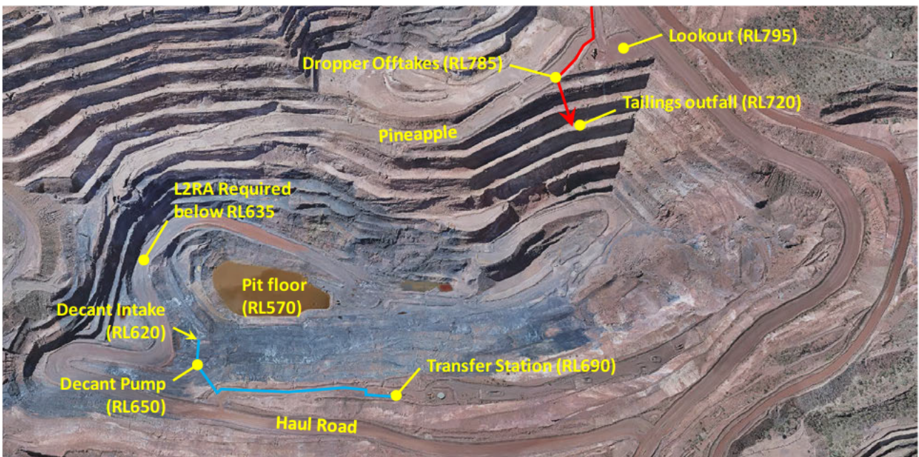
Figure 2-3 General Arrangement at SEP Pit
