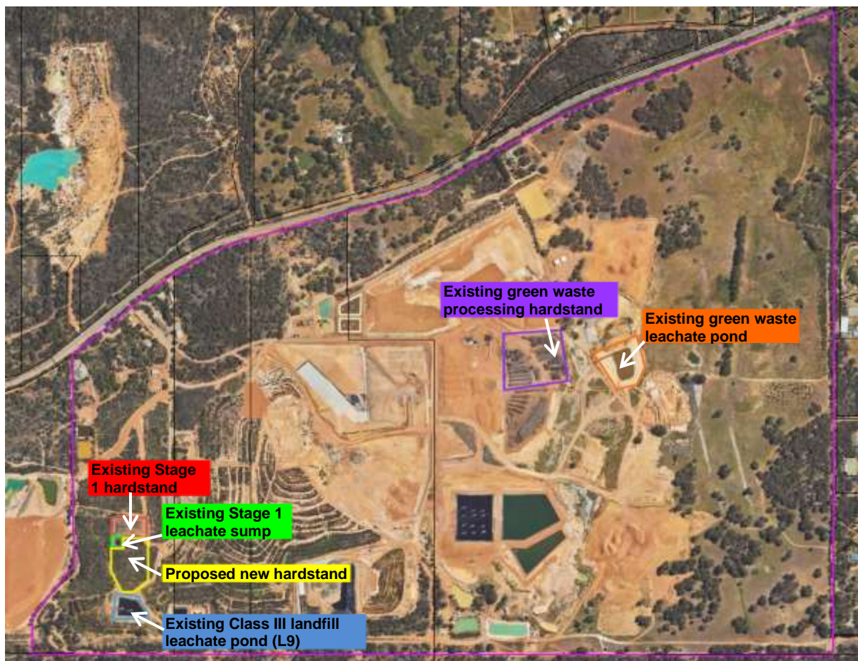
Figure 1: Layout of existing and proposed infrastructure for FOGO receipt, storage and processing
