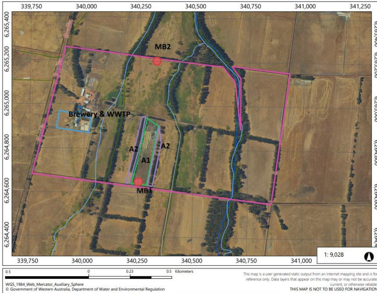
Figure 4. Monitoring Locations. A1 is the Irrigated paddock (outlined in green), A2 is the irrigated trees (outlined in purple), MB1 is the ungradient groundwater bore, MB2 is the down gradient monitoring bore (shown as red circles).
