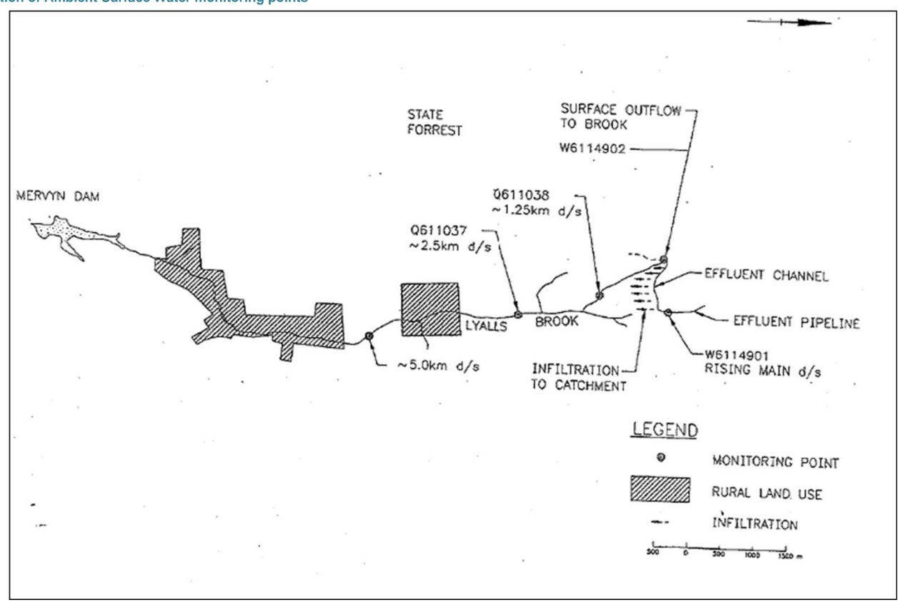
Location of Ambient Groundwater monitoring bores and infiltration channels
