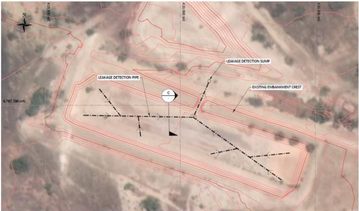
Figure 3: Vat leach dam – leak detection system location
