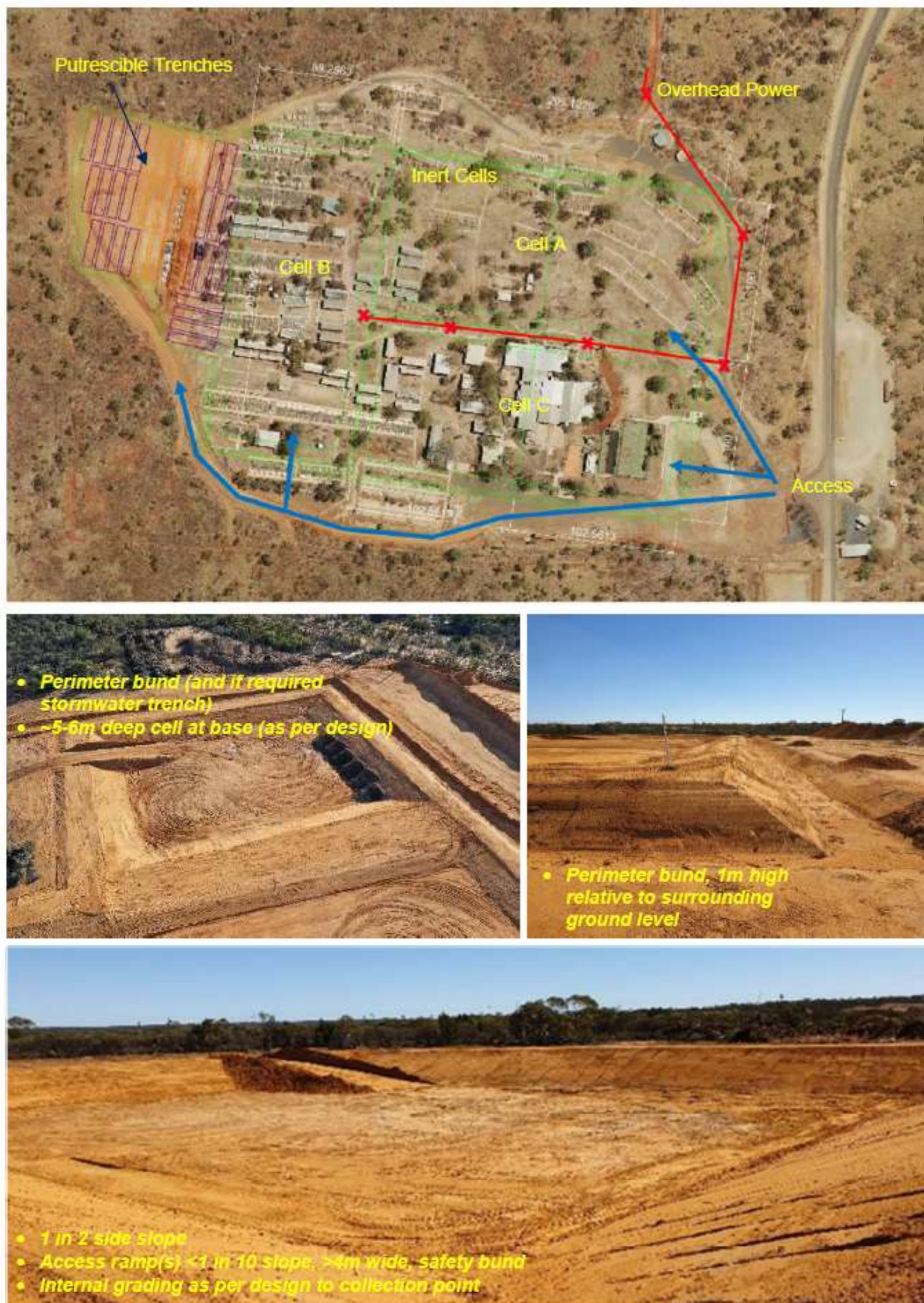
Figure 8: Primary landfill design
