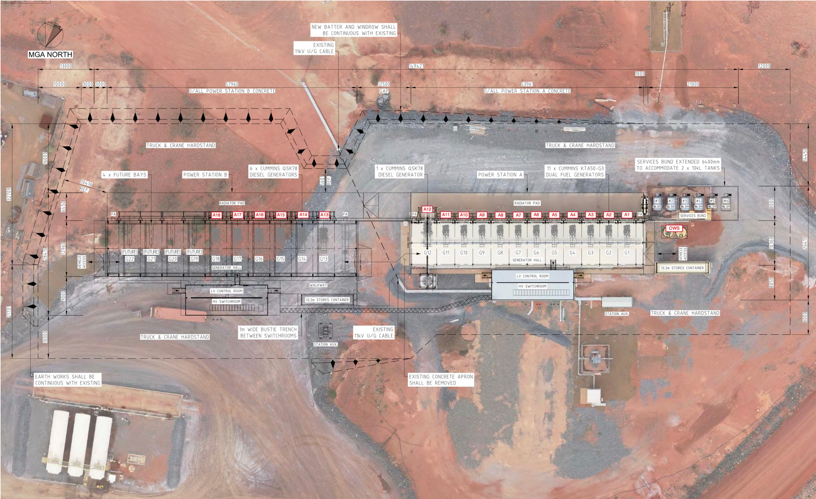
Figure 2: Layout of existing (Power Station A) and proposed (Power Station B) power station and discharge points
