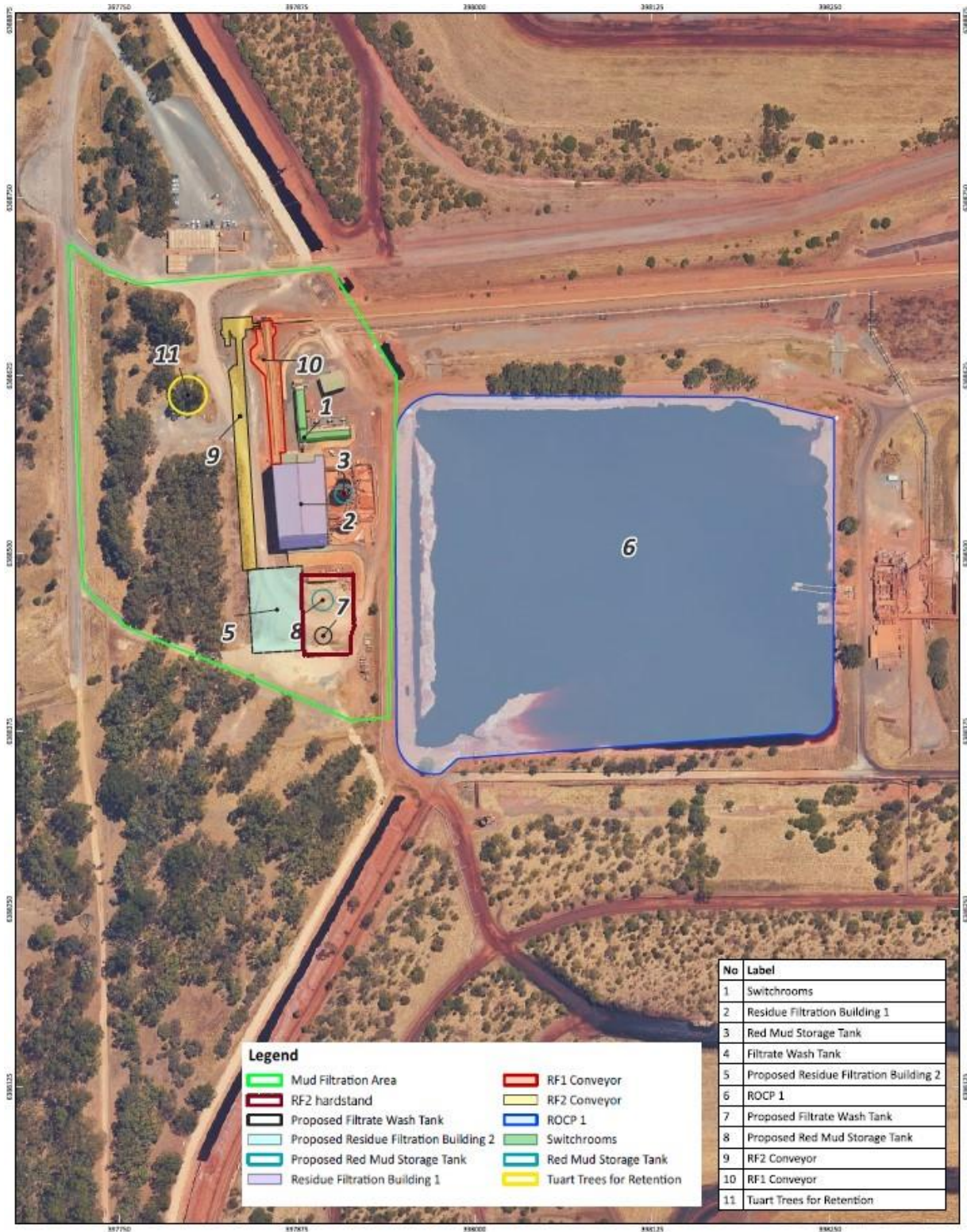
Figure 2: Residue Filtration Plant 2 site layout
