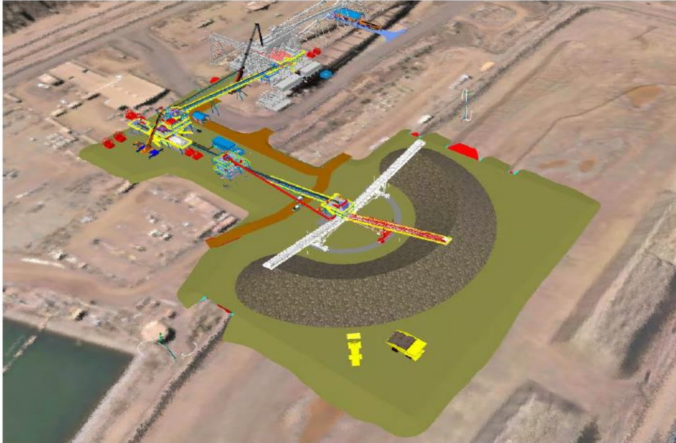
Figure 17: Indicative layout of proposed OPF1 Lump Plant
