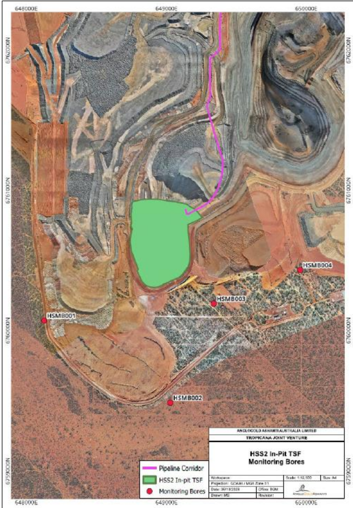
Figure 7: Location of HSS2 in-pit TSF groundwater monitoring bores (Table 6)
