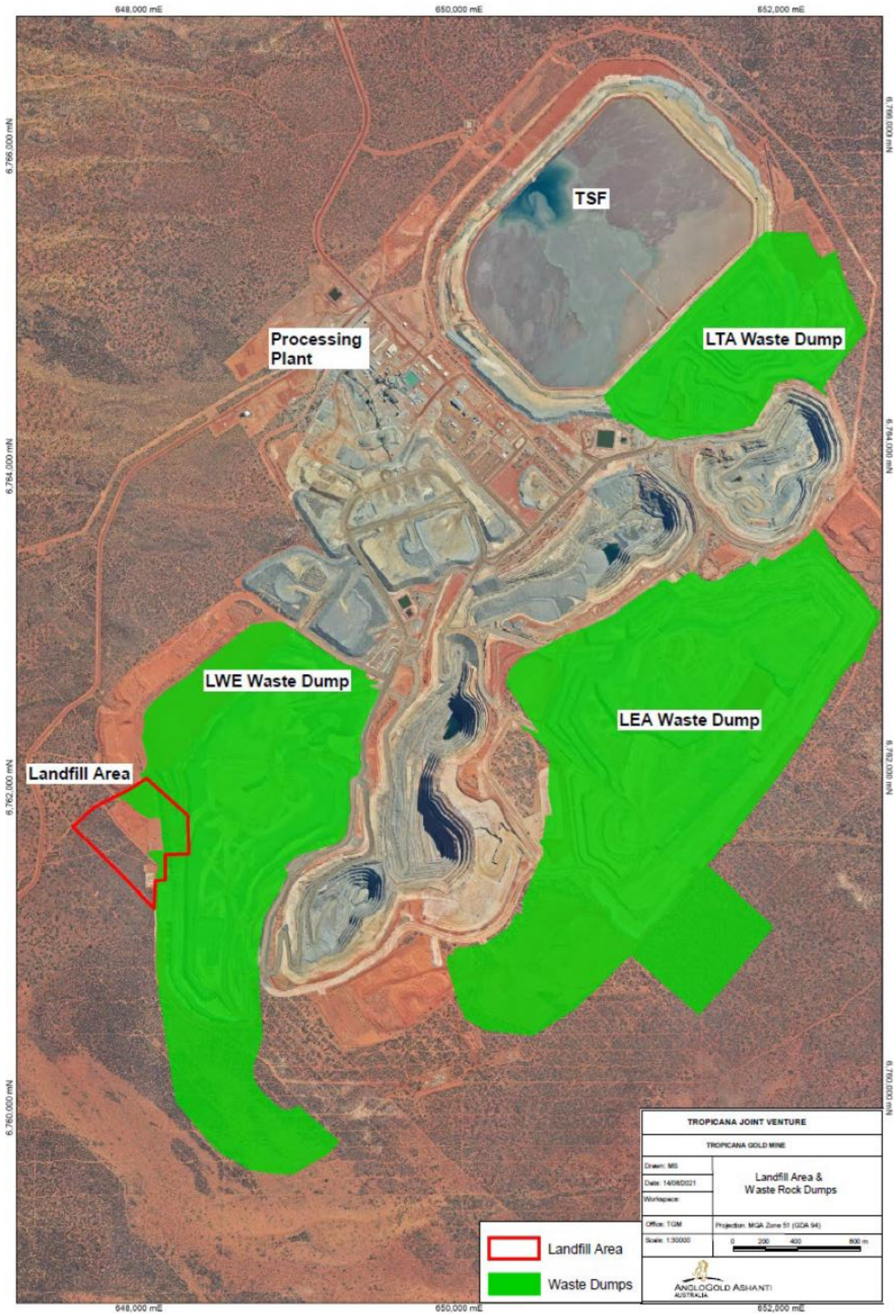
Figure 5: Overview of Premises. Note: does not show location of HSS2 in-pit TSF, see Figure 8
