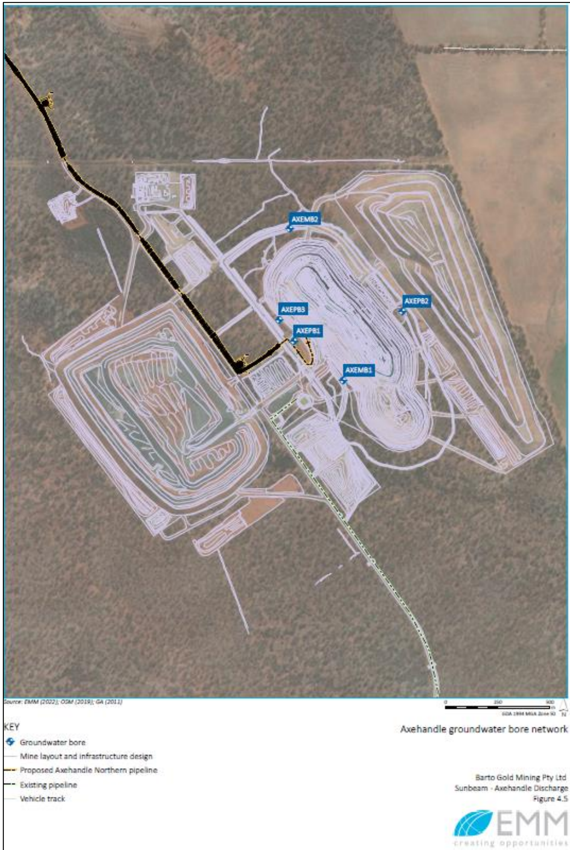
Figure 3: Location of existing monitoring bores defined in Table 11, condition 38 surrounding Axehandle Pit
