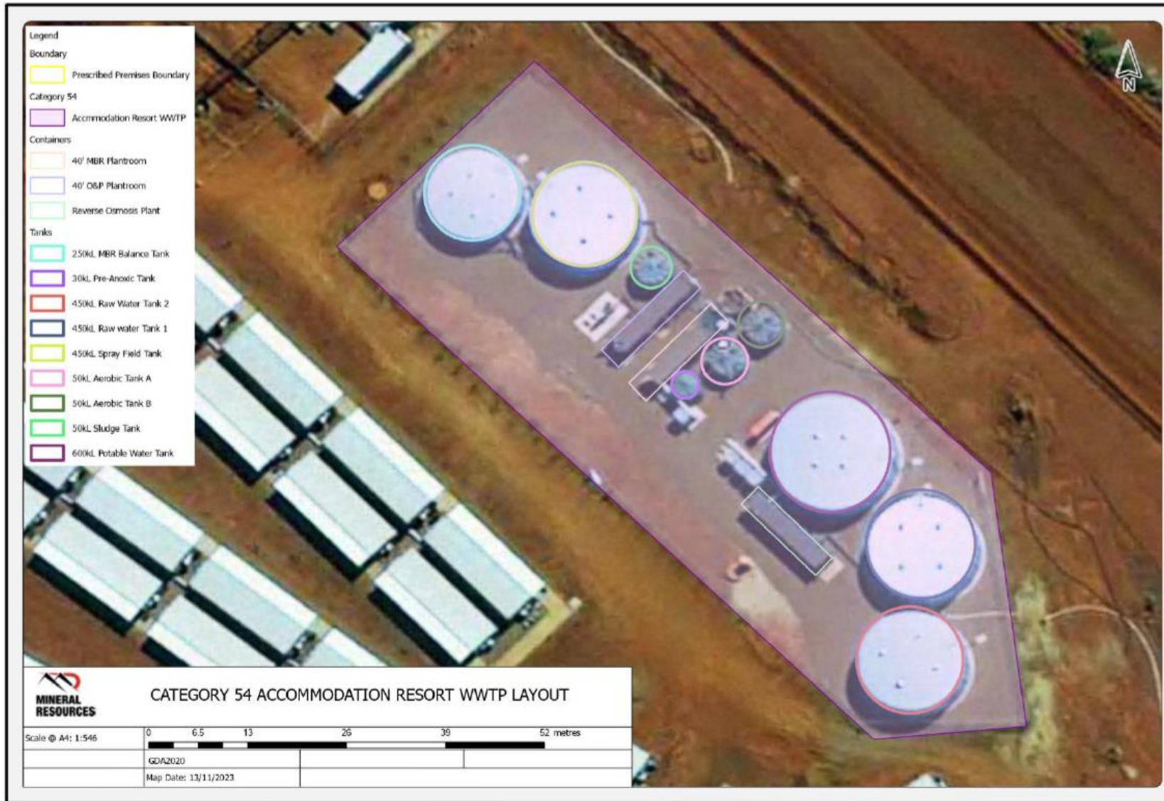
Figure 5: Layout of Accommodation Resort WWTreatment Plant (200 m 3 /day)
