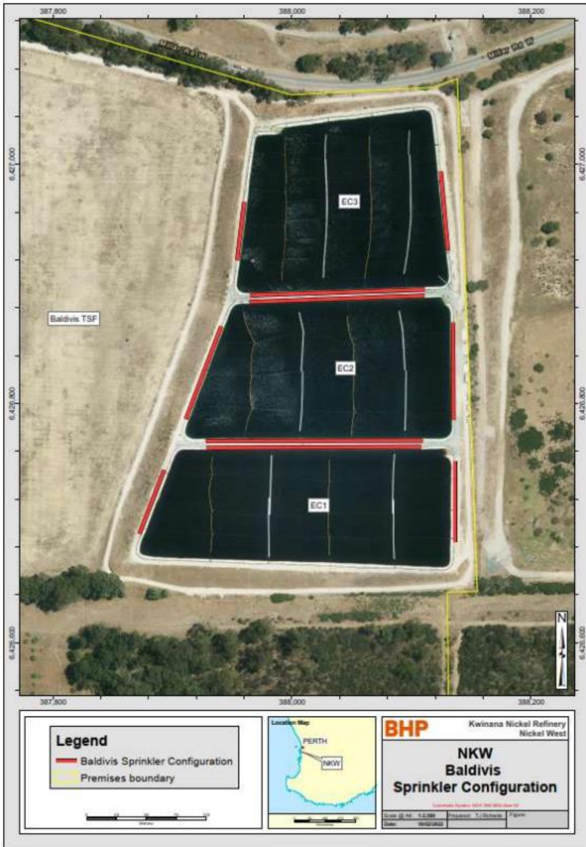
Figure 5: Baldvis facility: evaporation cells 1, 2 and 3 Sprinkler locations
