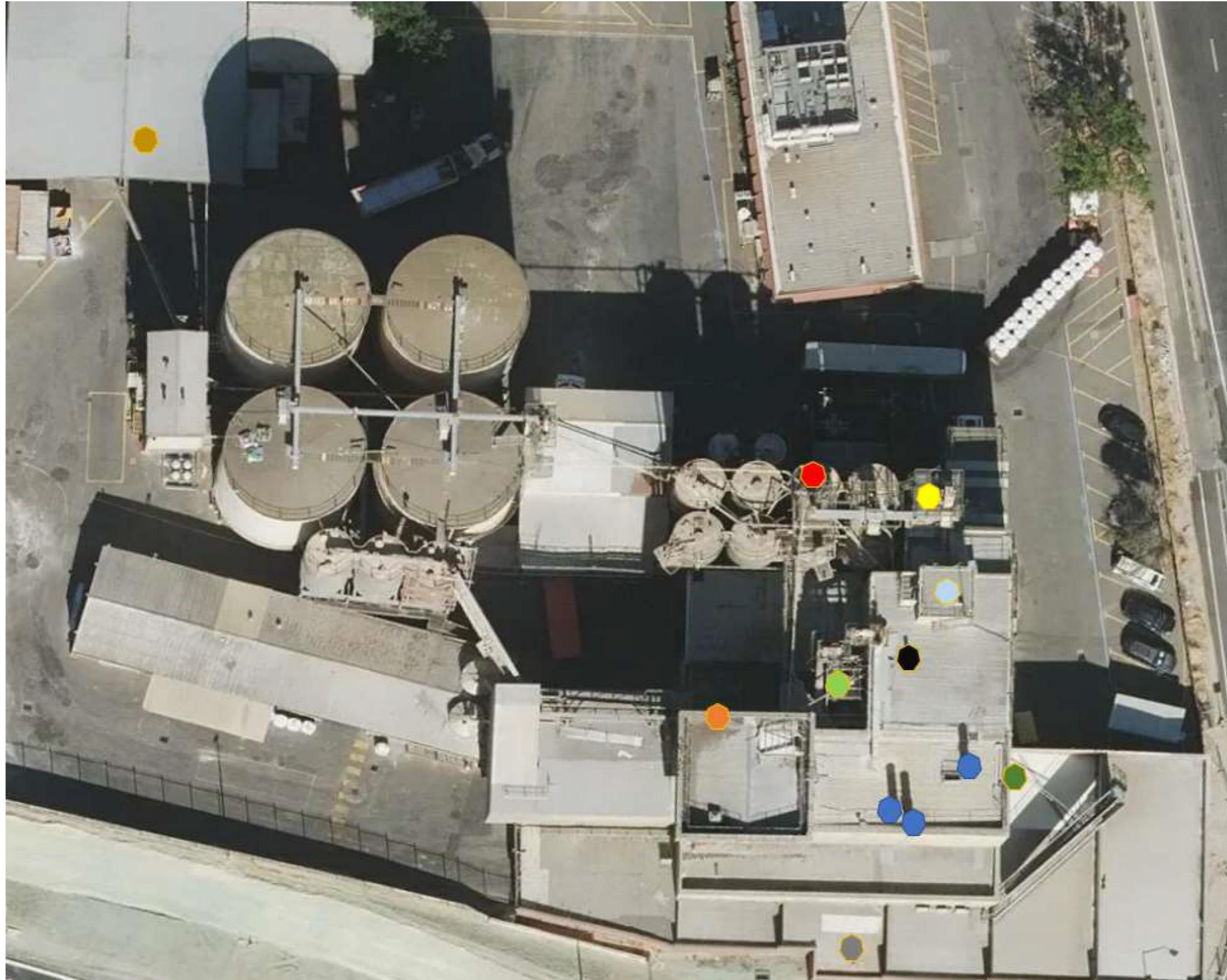
Figure 5: Dust filter and cyclone emission points
