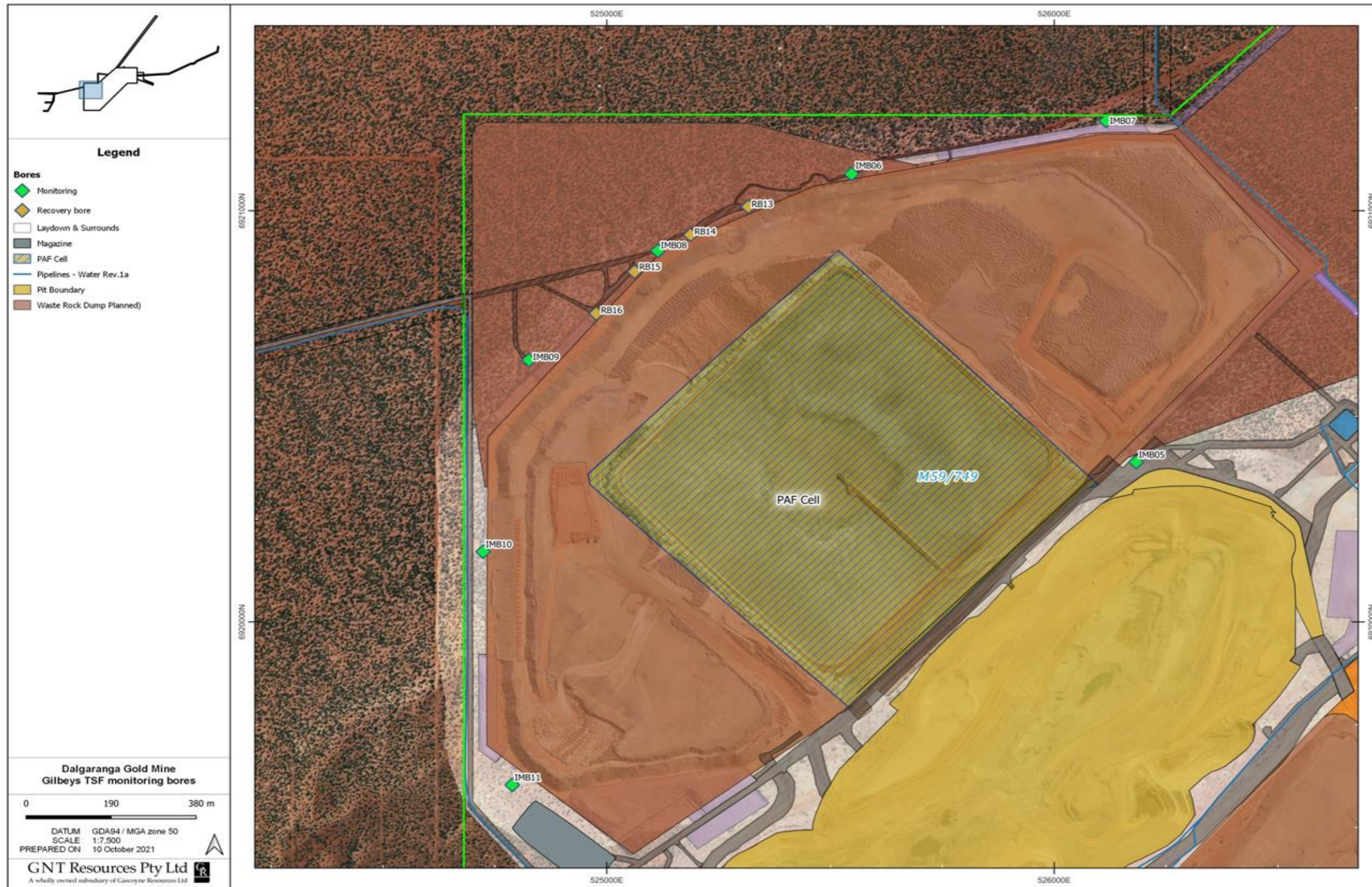
Figure 4: Gilbeys TSF groundwater monitoring bores
