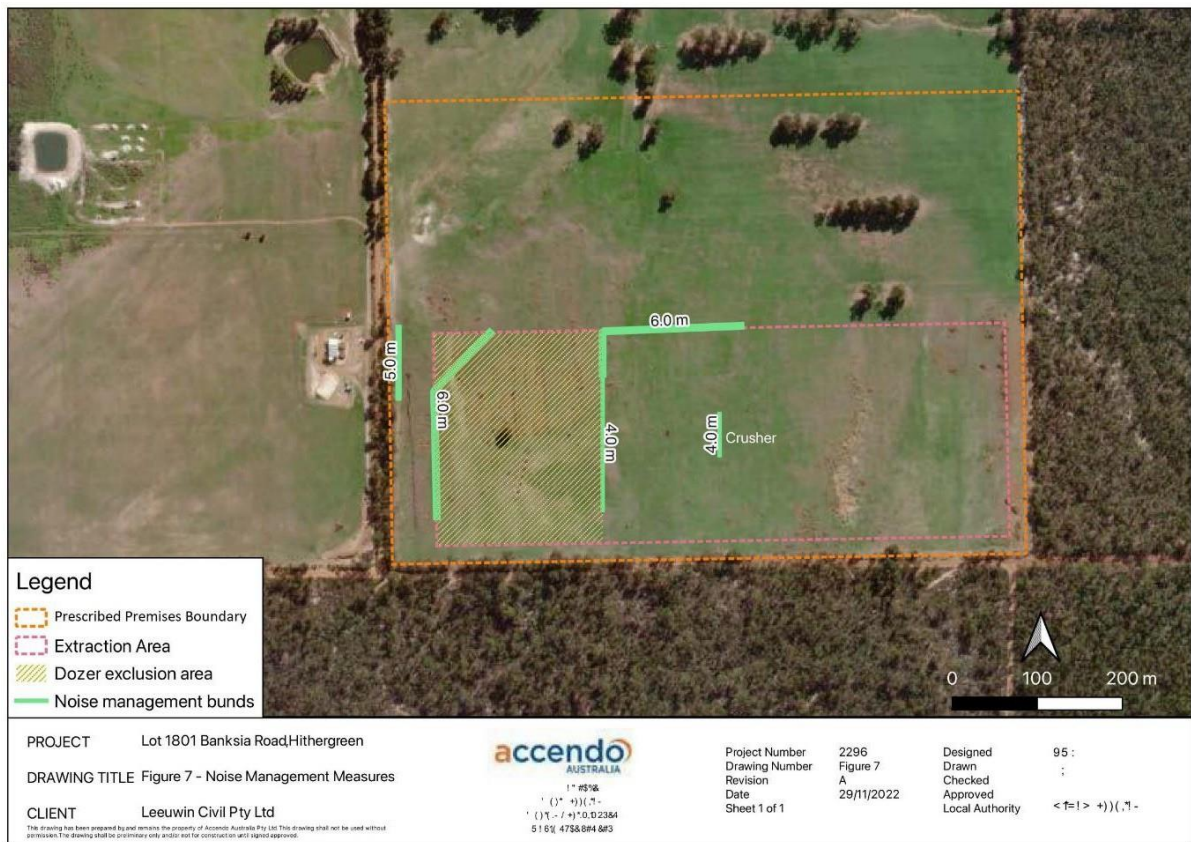
Figure 1: Map of the boundary of the prescribed premises with noise bund construction requirements and dozer exclusion area
