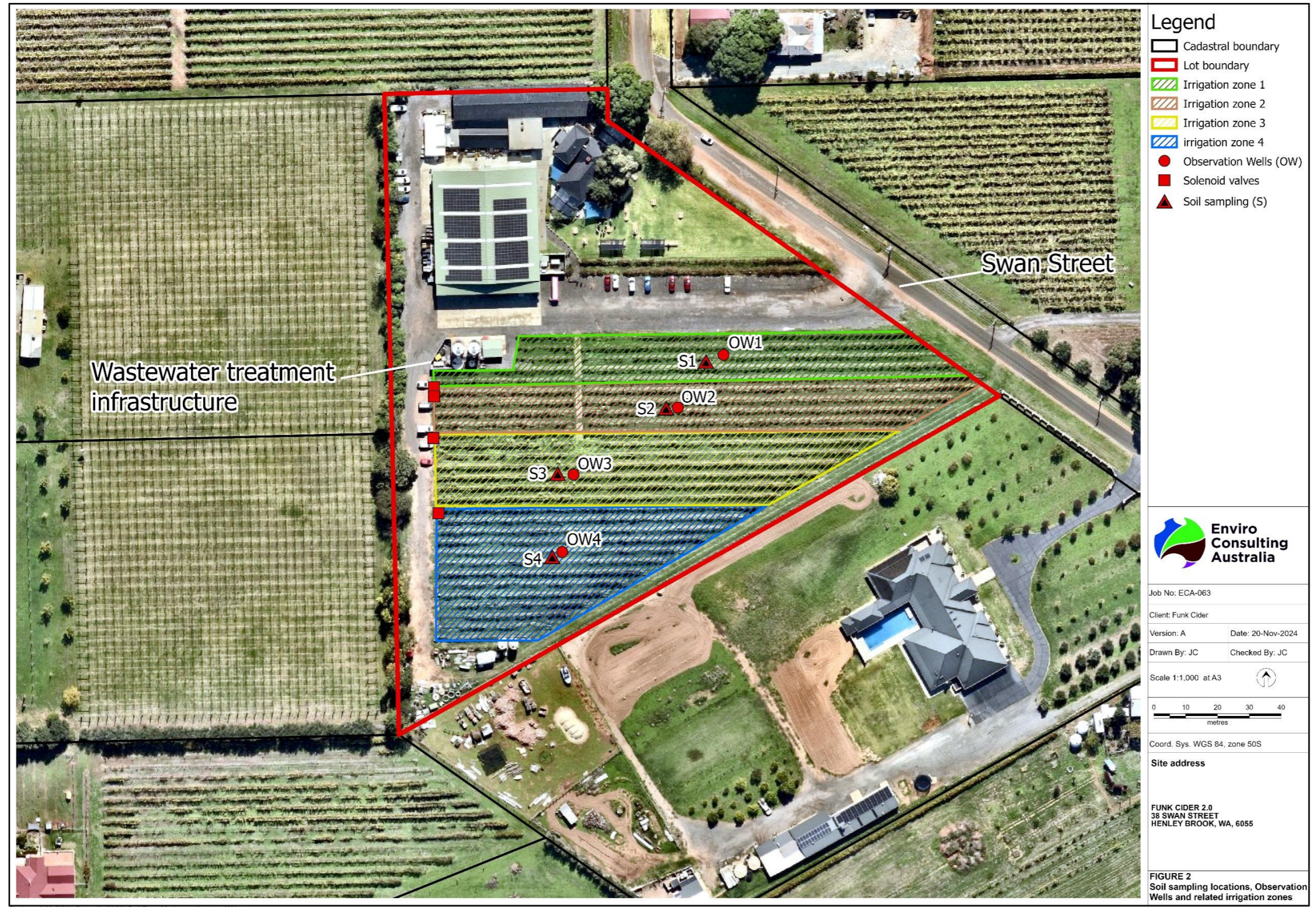
Figure 2: Observation Wells (OW) used for soil saturation monitoring within each irrigation zone
