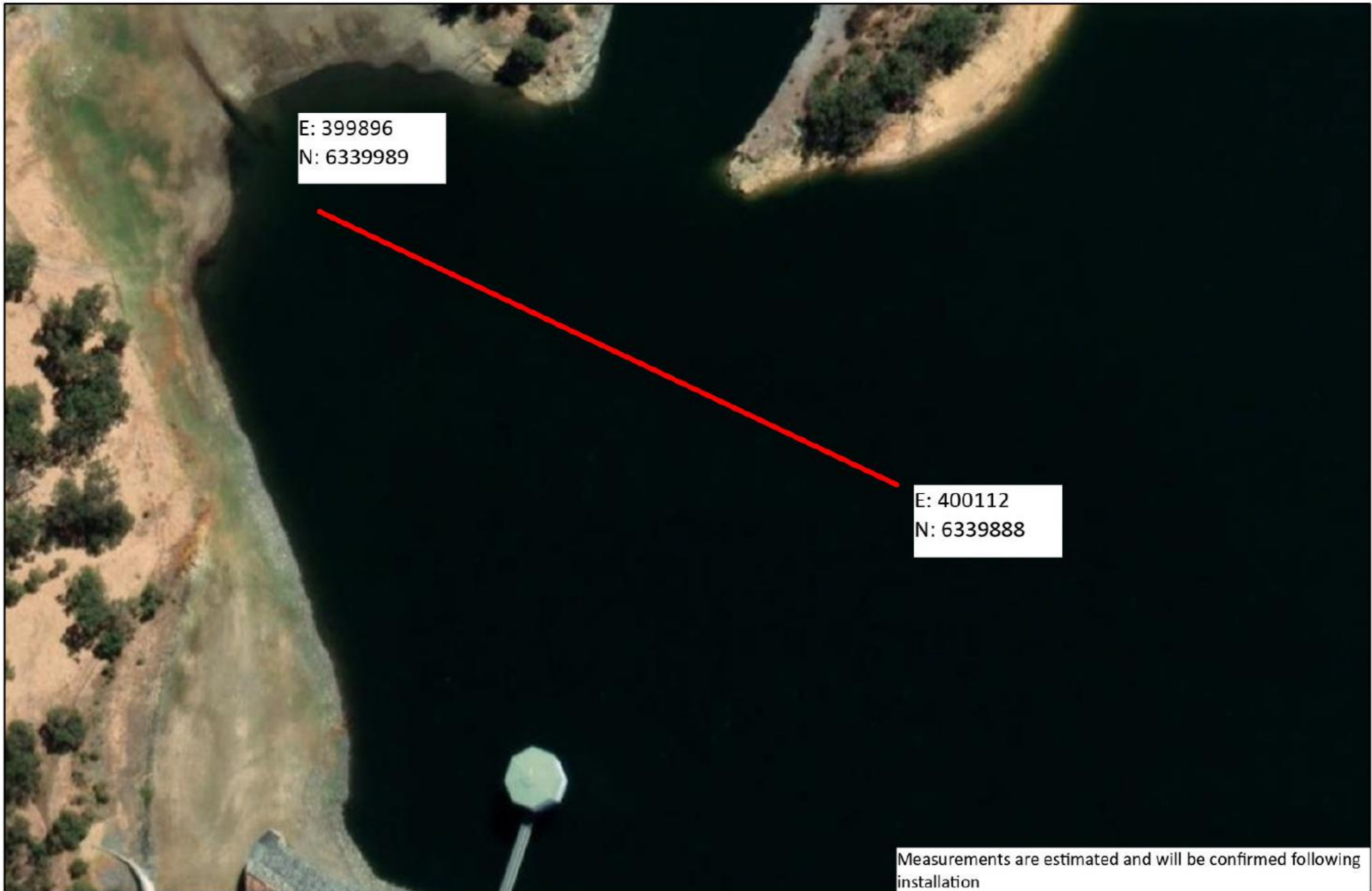
Figure 2: Pipeline route and diffuser location
