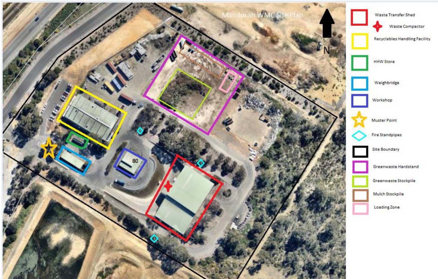
Figure 2: Gordon Road transfer station site plan.
