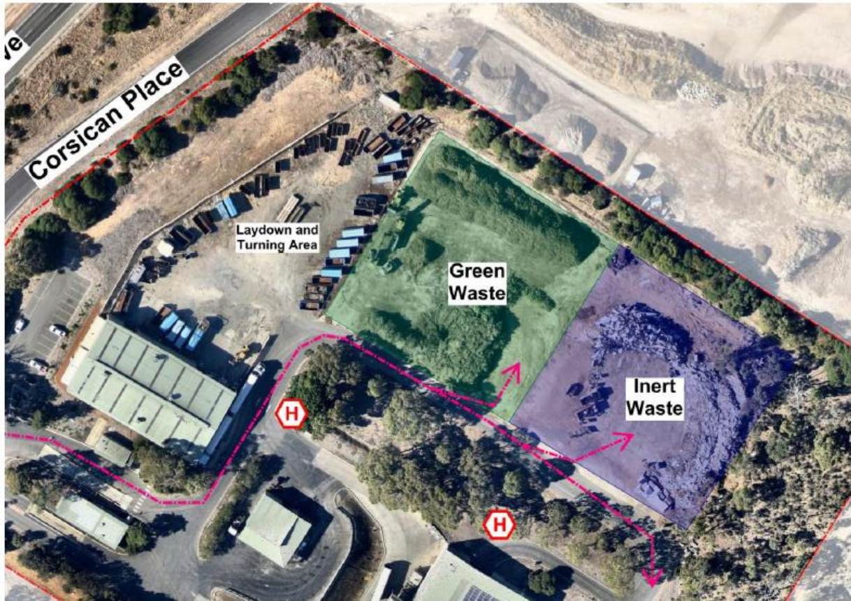
Figure 5.1 - Bulk Waste Area Layout – Existing Hydrant Provisions
