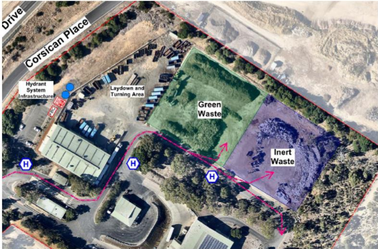
Figure 5.2 - Bulk Waste Area Layout – Upgraded Hydrant Provisions
