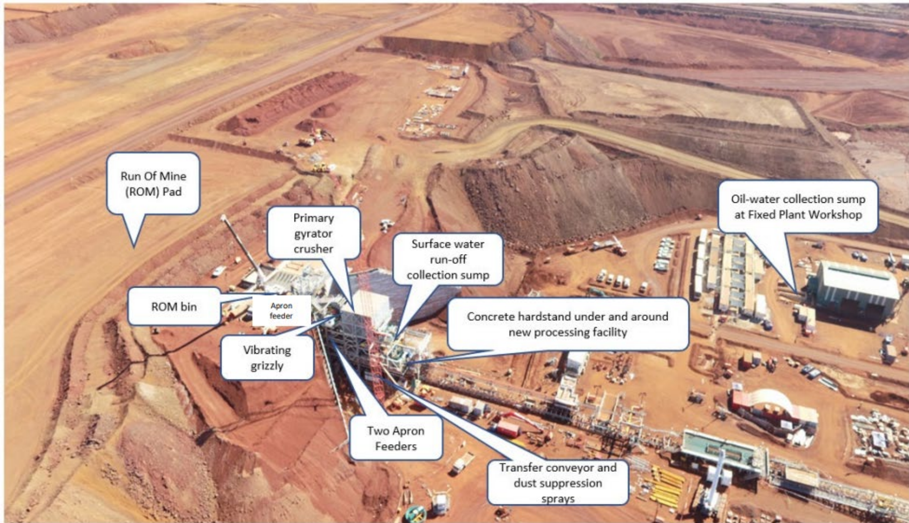
Figure 12: WTS S2 Processing Facility layout
