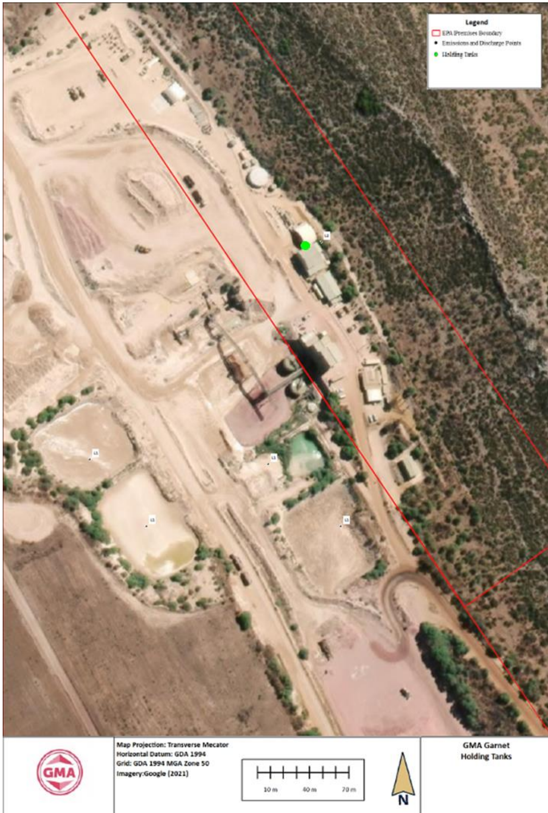
Figure 3: Holding tanks and emission and discharge points
