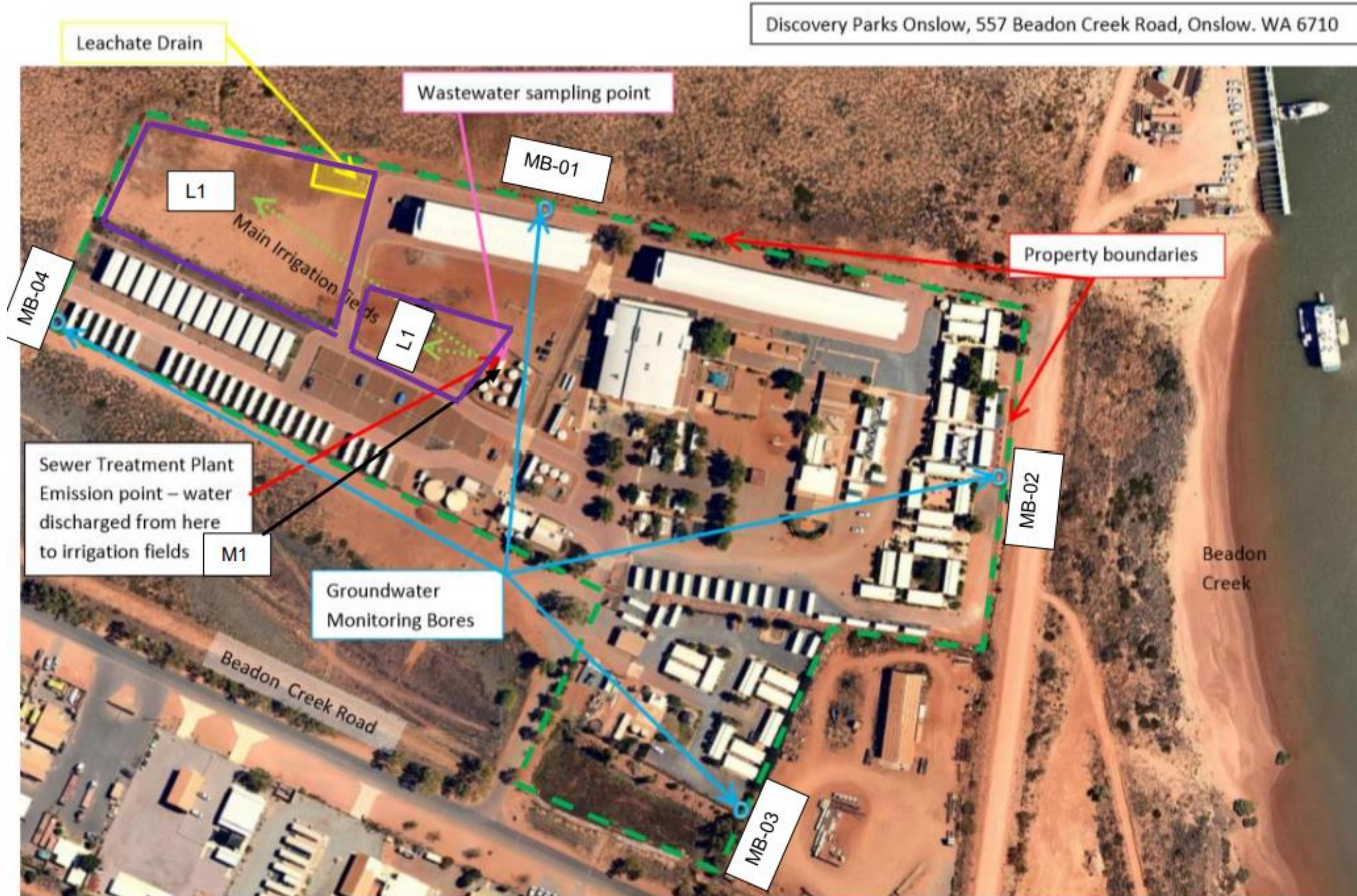
Figure 2: Emission and monitoring point locations
