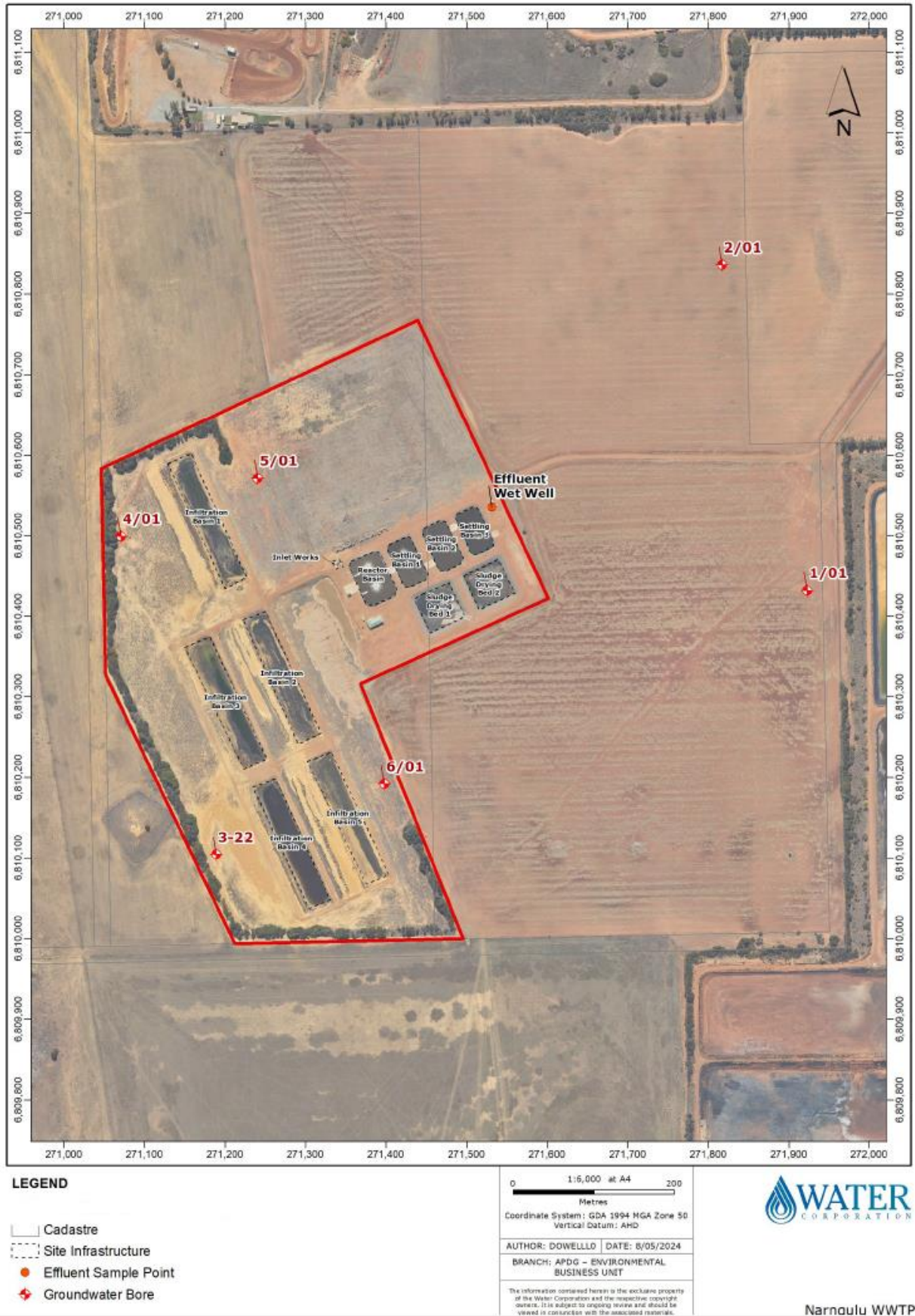
Figure 4: Groundwater monitoring bore network
