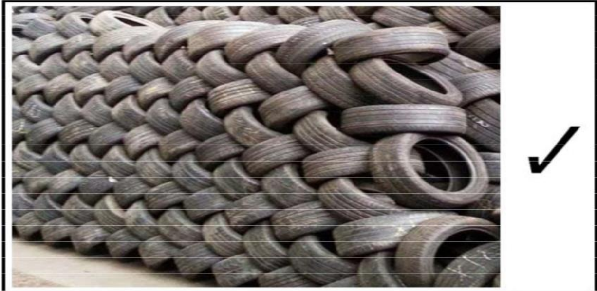
Figure 4: Laced storage of tyres.
