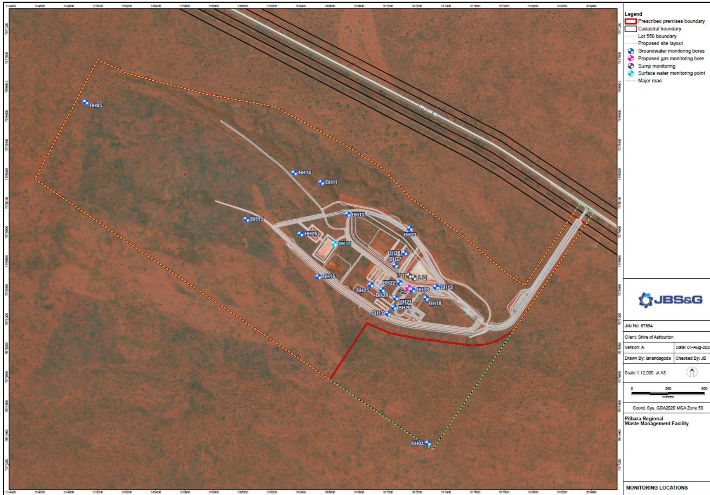
Figure 3: Monitoring bore locations.
