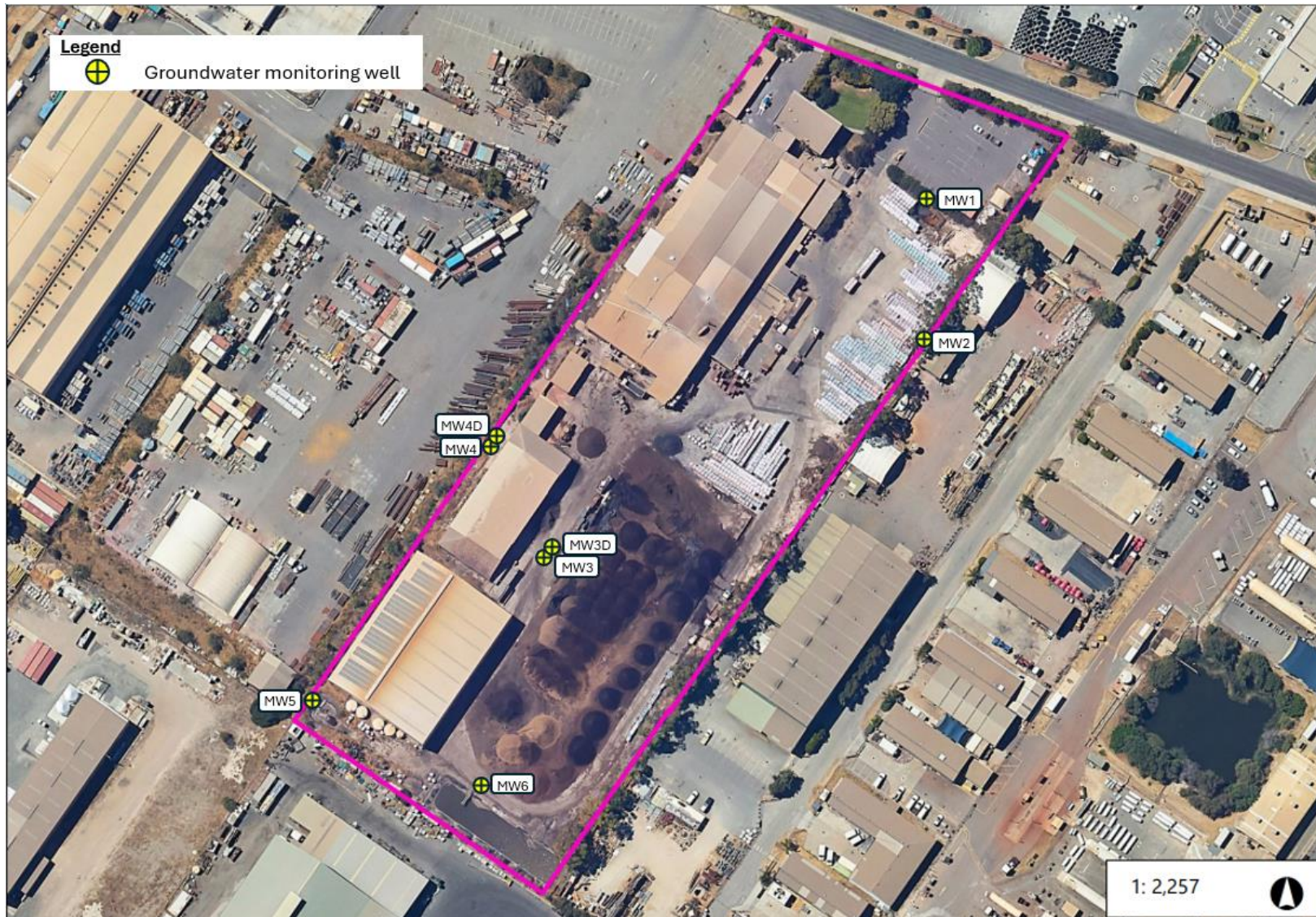
Figure 4: Map of proposed new groundwater monitoring well locations
