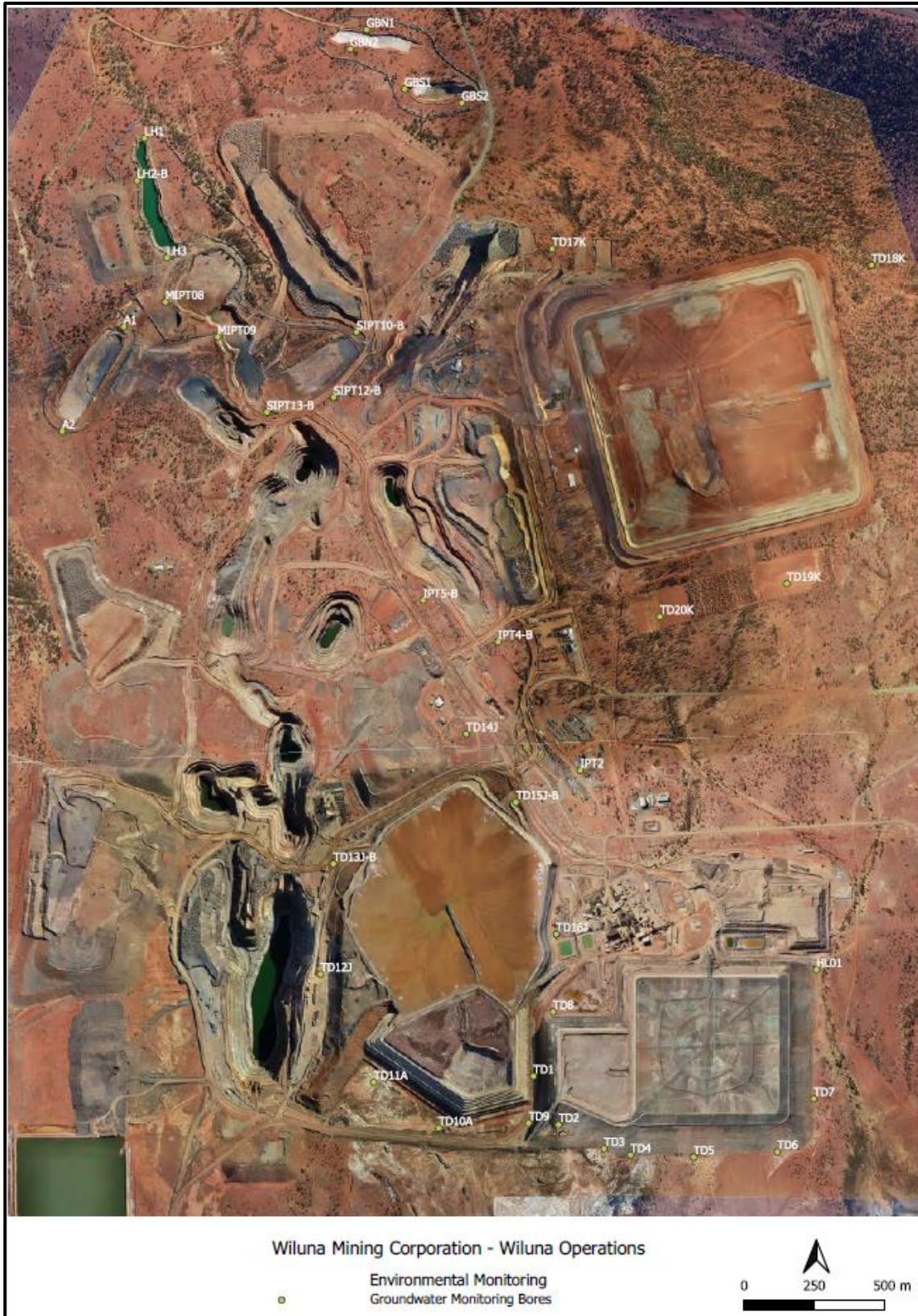
Figure 5. Environmental ambient groundwater monitoring bores and process monitoring points
