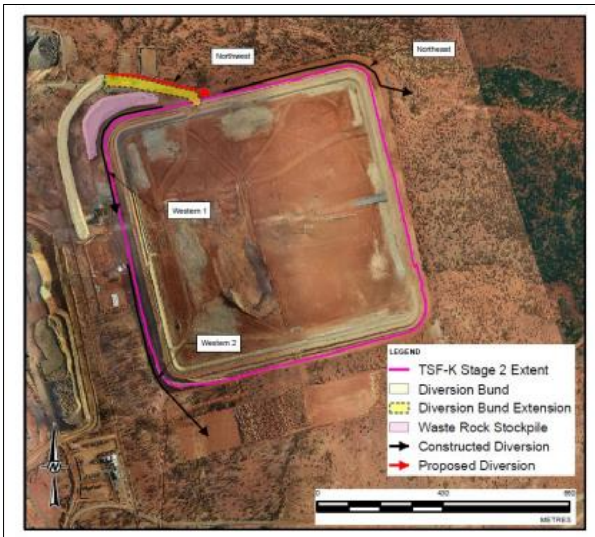
Figure 8: Map showing location of diversion drain alignments for TSF K Stage 2 embankment raise
