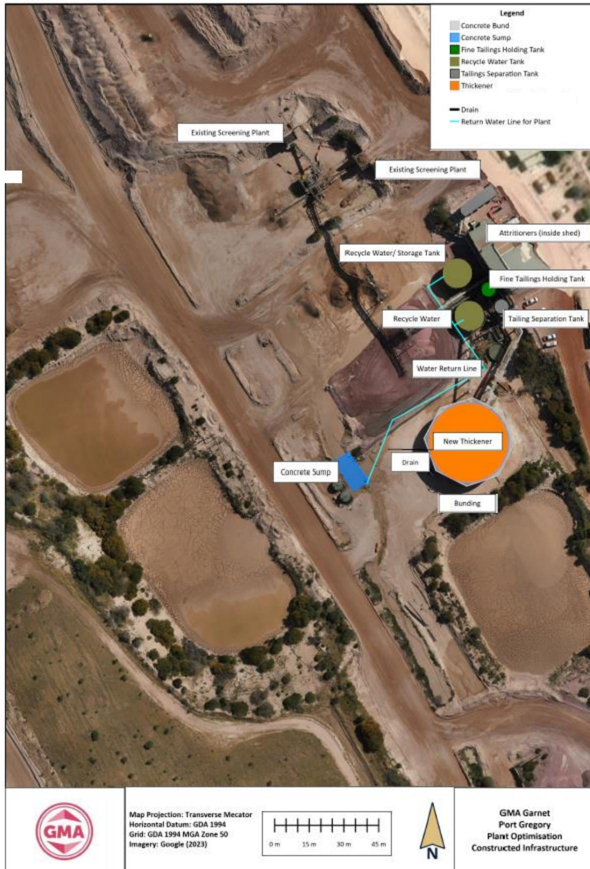
Figure 3: Process plant layout
