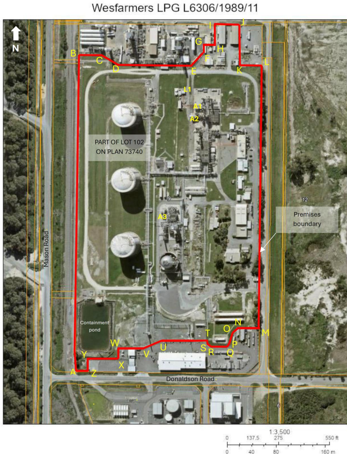
Figure 1: Map of site layout and emissions and discharges (air and land) and monitoring location (air)
