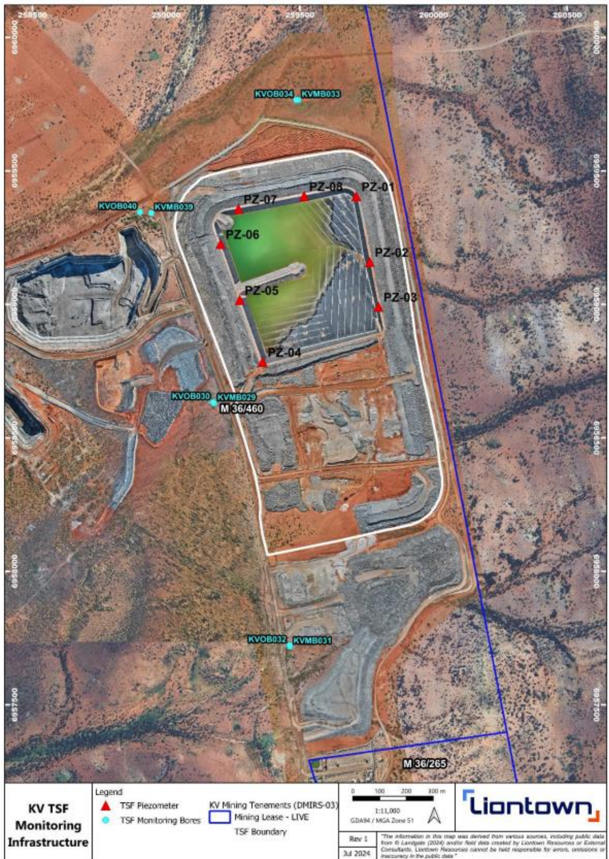
Figure 3: Locations of groundwater monitoring bores and VWPs
