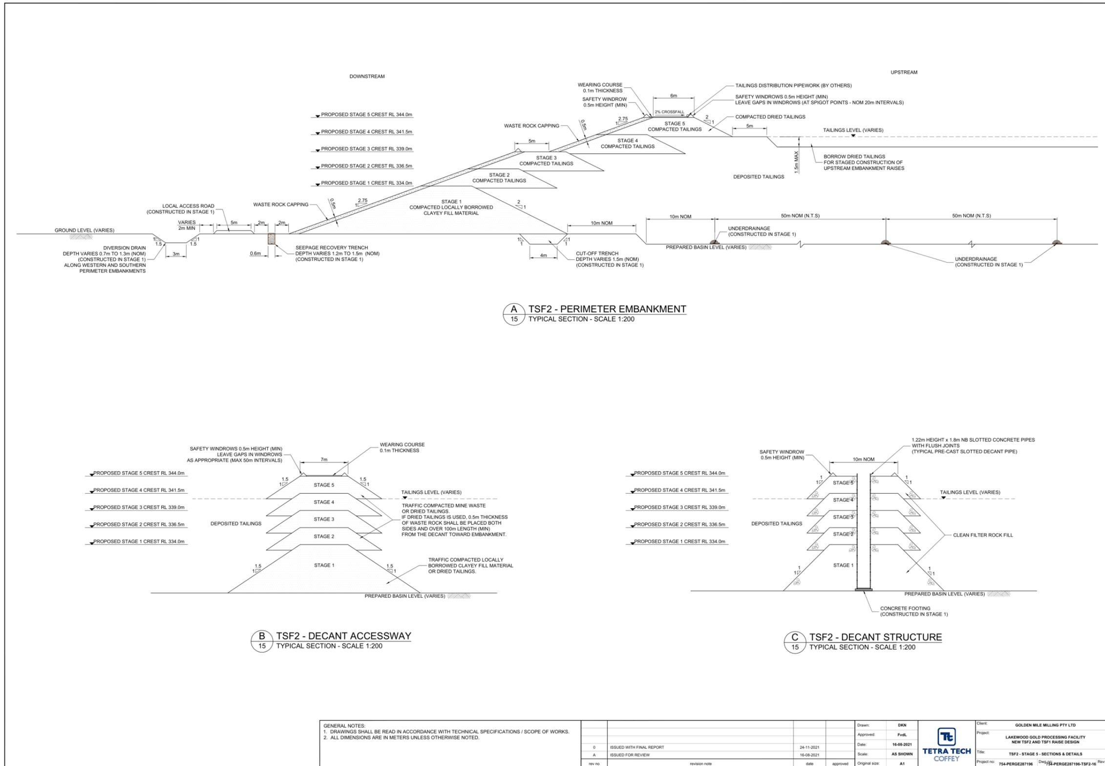
Figure 9: TSF2 – Stage 2 to 3 construction drawings
