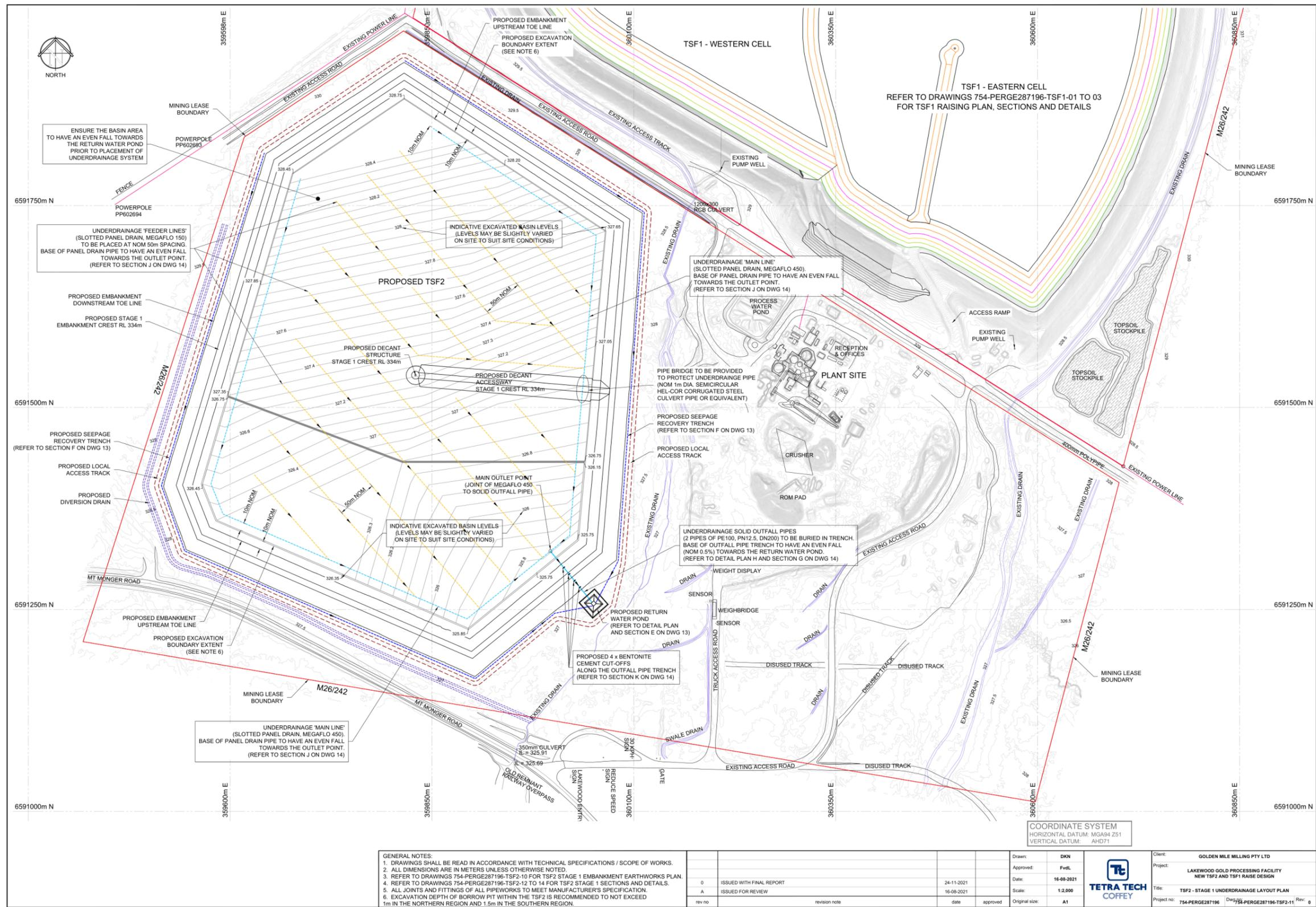
Figure 12: TSF2 – Underdrainage system construction drawing
