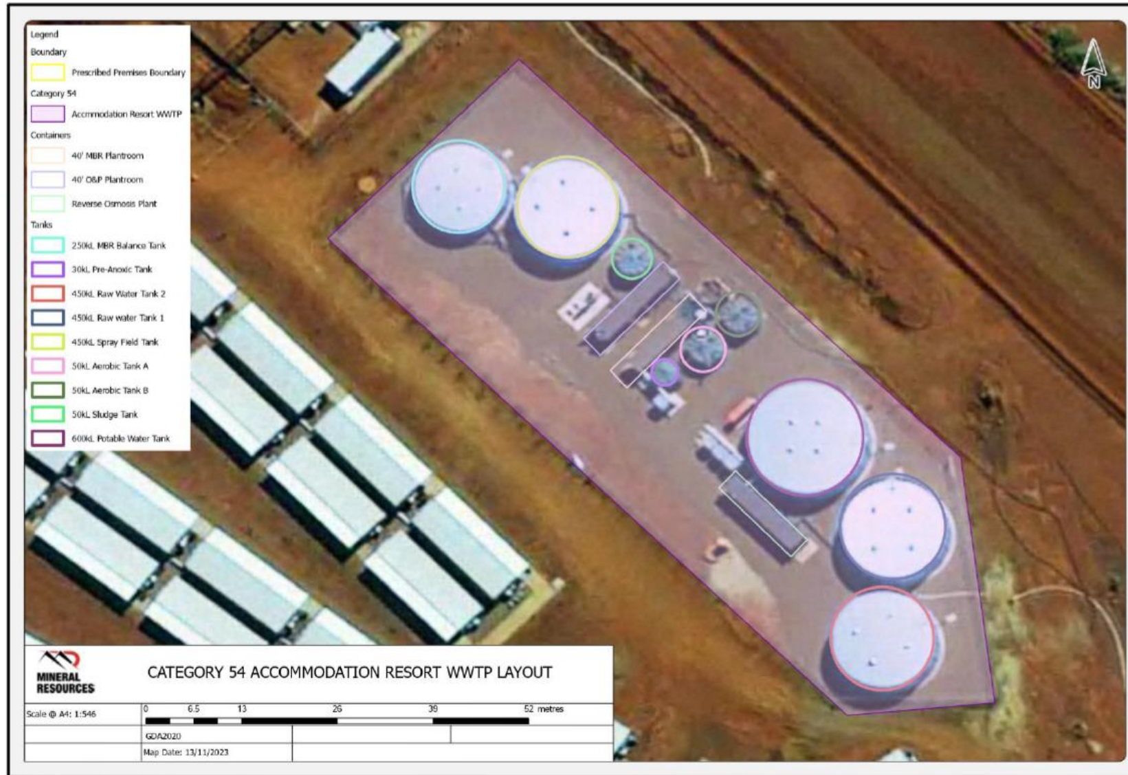
Figure 6: Layout of Accommodation Resort WWTP (200 m 3 /day)
