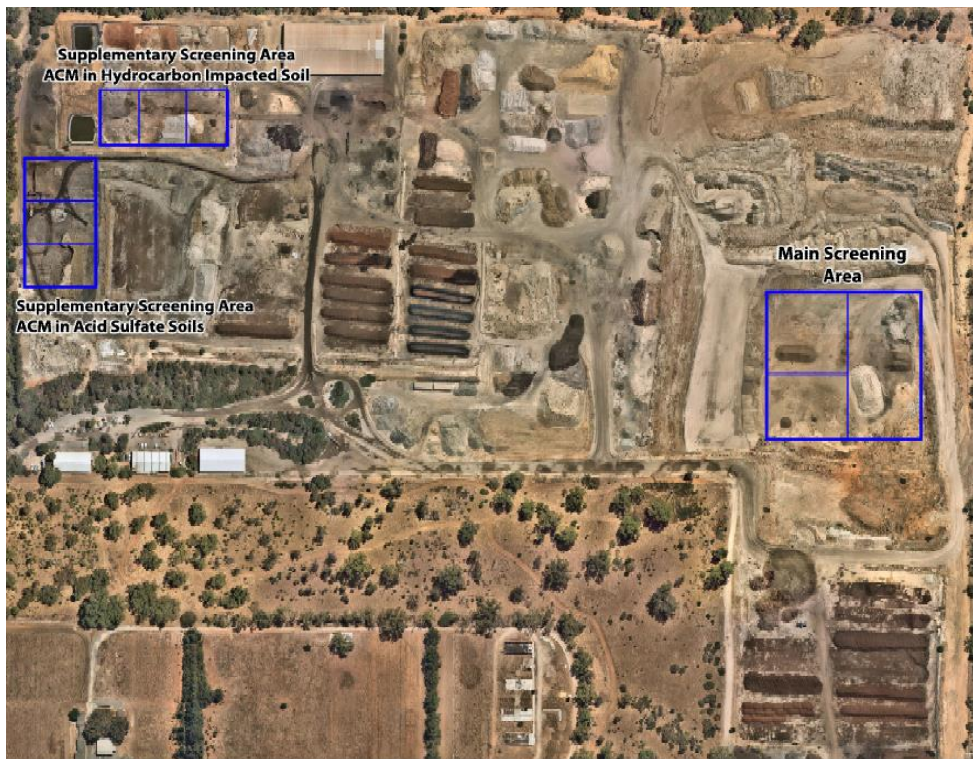
Figure 2: Overview of asbestos or ACM contaminated soil screening areas
