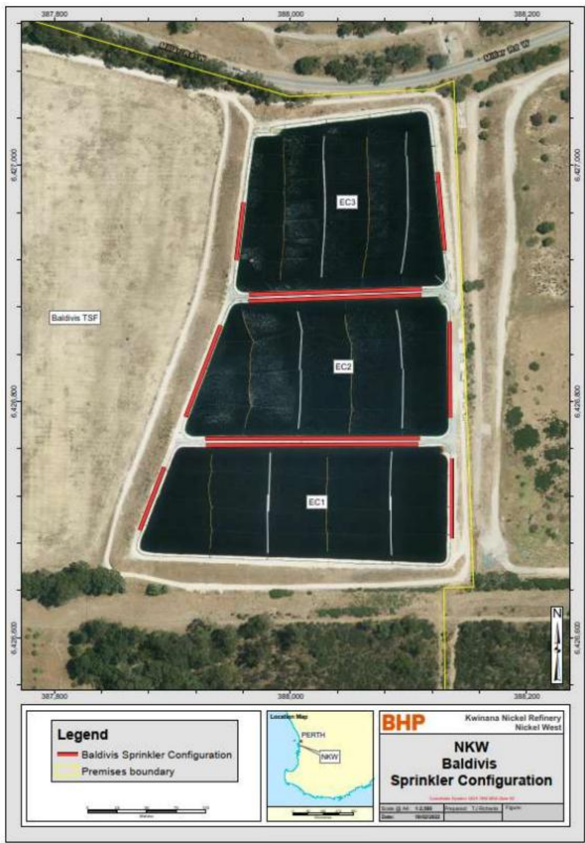
Figure 5: Baldivis facility: evaporation cells 1, 2 and 3 Sprinkler locations
