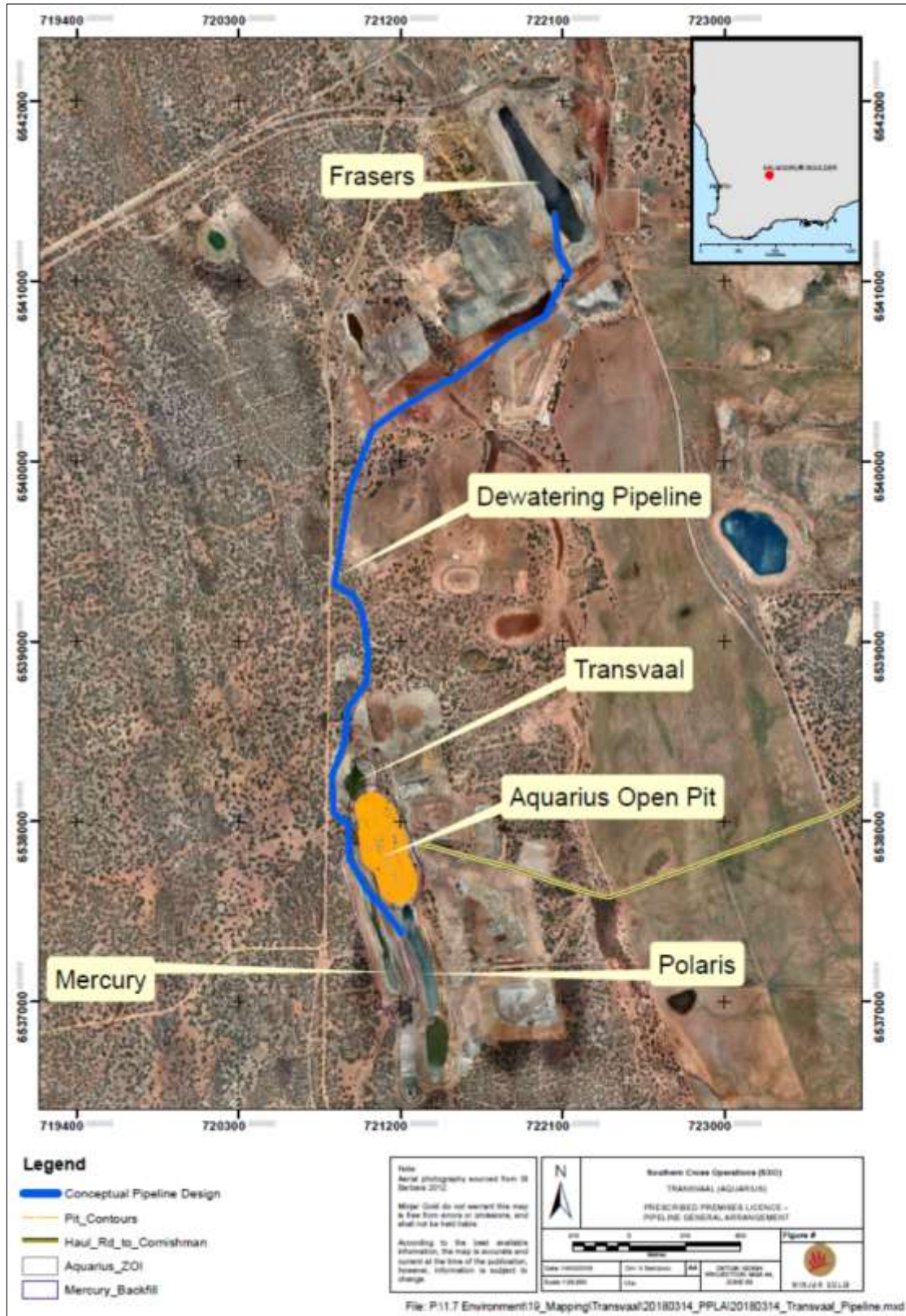
Figure 12: Dewatering pipeline from Frasers to the Transvaal complex
