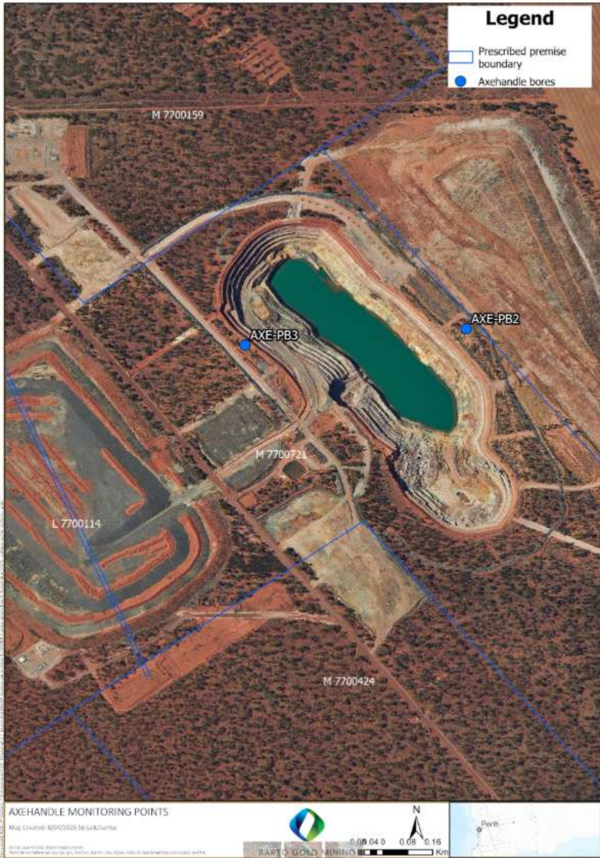
Figure 5: Location of existing monitoring bores defined in Table 13, Condition 39 surrounding Axehandle Pit
