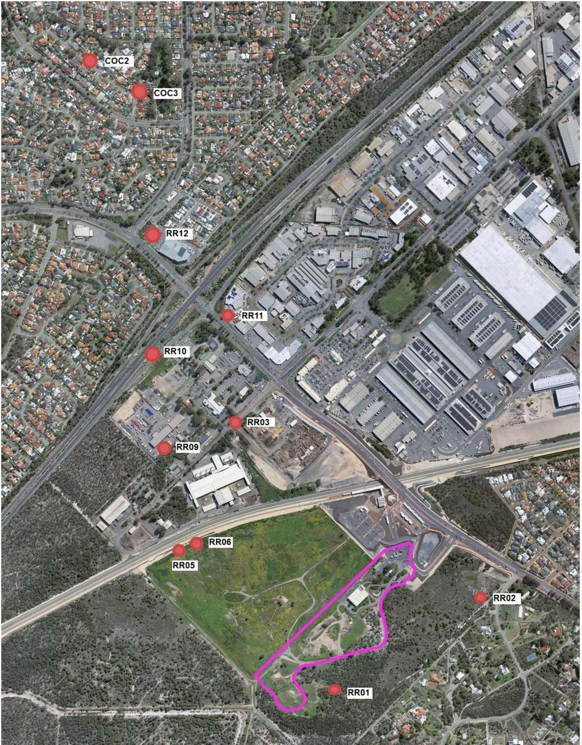
Figure 3: Groundwater monitoring bore locations
