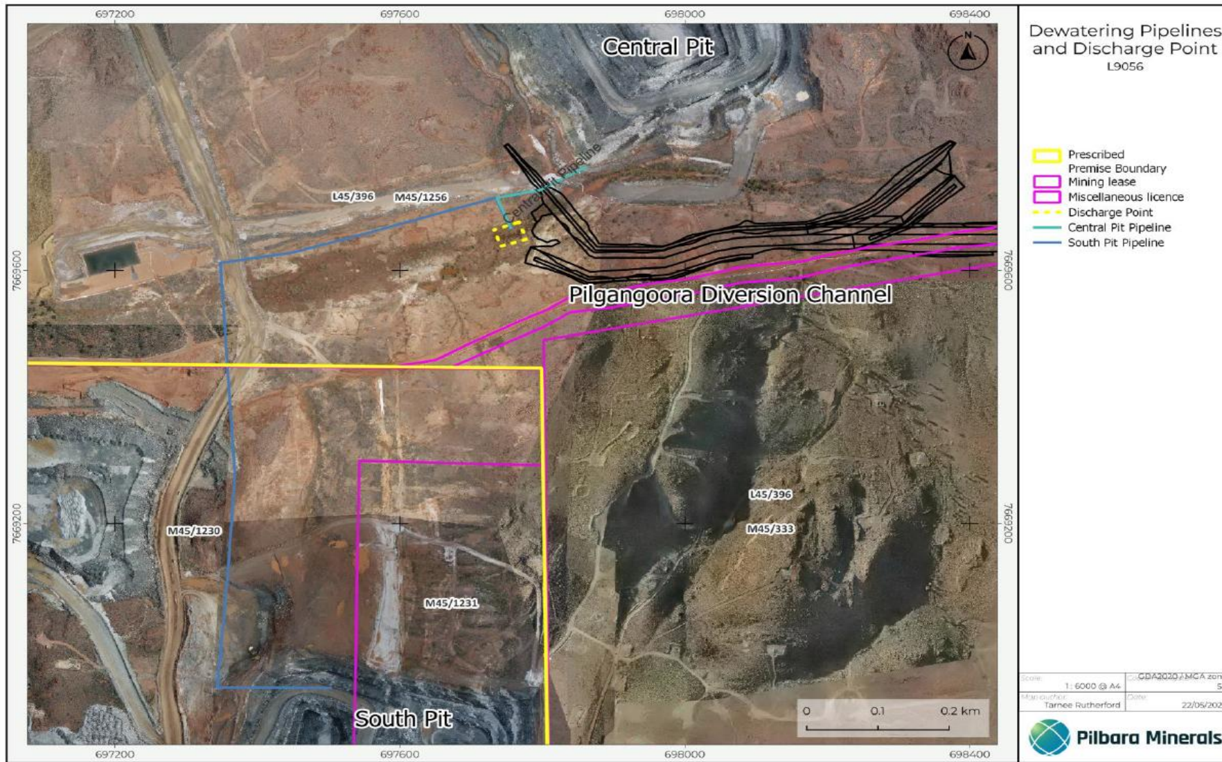
Figure 9: Pilgangoora Creek discharge point and location of off-site “south pit” and central pit pipelines.
